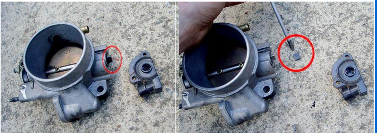
Make sure to save the plastic square sleeve that slides off the shaft end (circled in red).
