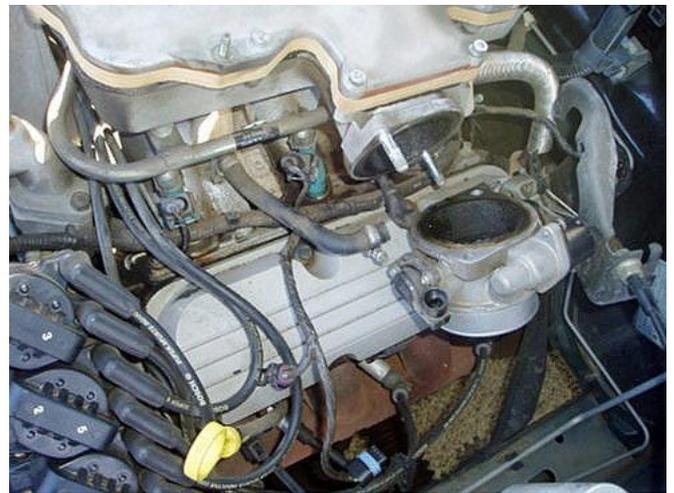
**Step 10** – Hold the rubber elbow & pull it off the tube (circled above).
