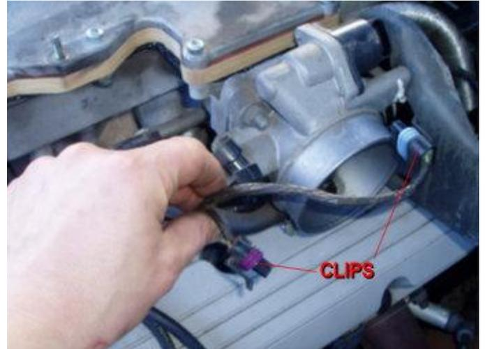
**Step 6** - Loosen the small hose clamp on the hose running to the front of the throttle body, & remove the hose from the throttle body.
