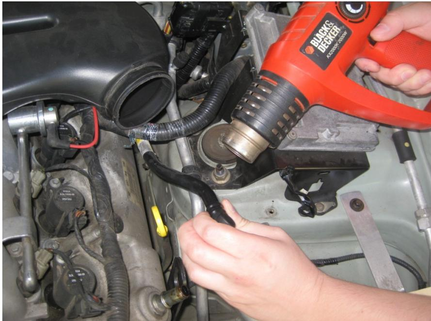
Counter the bend with your hands and refit the hose onto the nozzle making sure there is still enough clearance between the PCV hose and the oil dipstick. Refit the intake hose and check clearance. Adjust PCV hose further if required.
