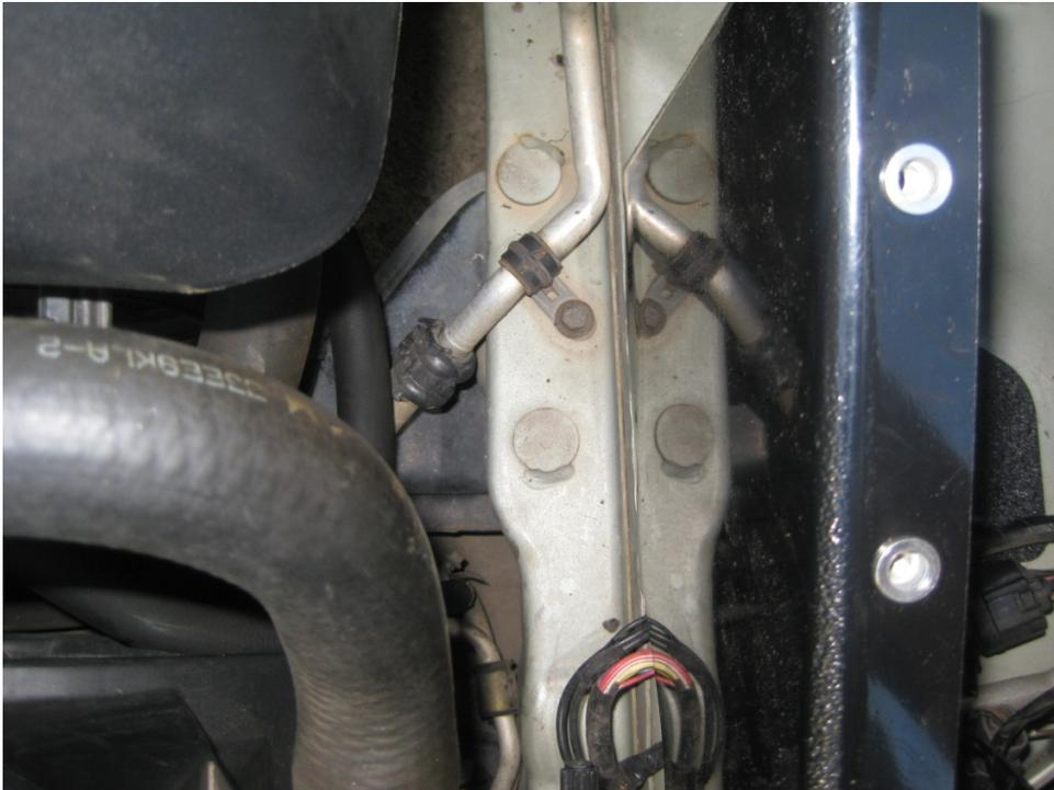
Use the flat straight bracket (provided) and one of the vehicle's original bolts in order to secure the base of the enclosure.
