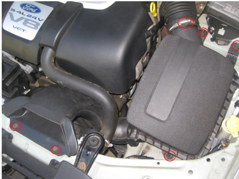
Start by loosening the hose clamp on the hose which connects to the lid of the air box.
