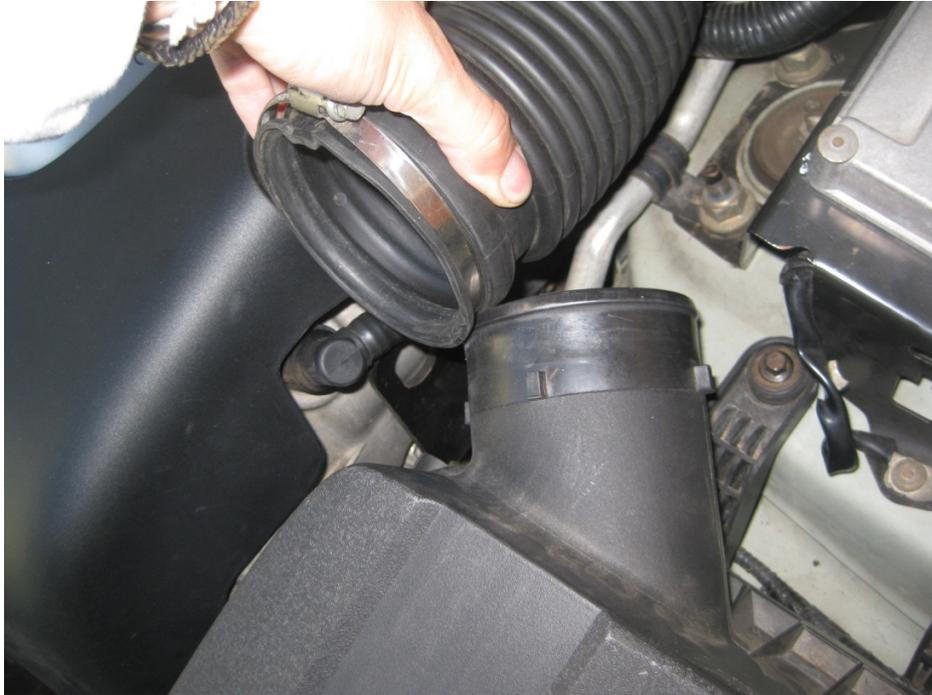
Proceed by removing the two screws on the intake snorkel as shown below
