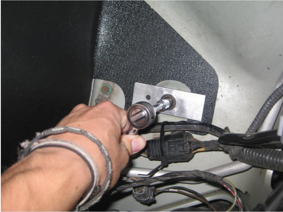
The enclosure should also be mounted at the top using the existing outer hole in the bodywork and the L-shaped bracket provided.
