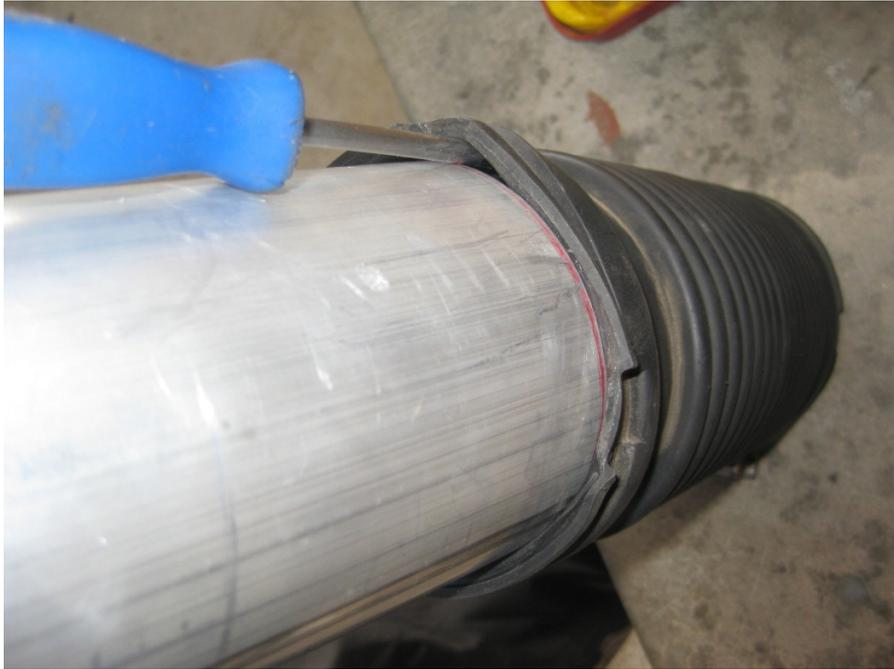
Secure the tube using the original hose clamp
