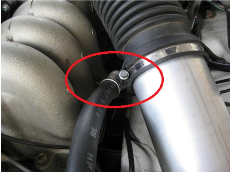
Carefully push down onto the A/C line in order to alter its angle and increase clearance.
