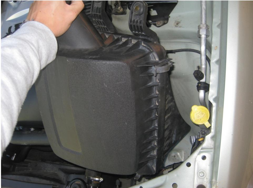
Also remove the washer bottle lid to allow for easy installation of the CAI. Once the CAI is fitted, the washer lid will need to be placed back.
