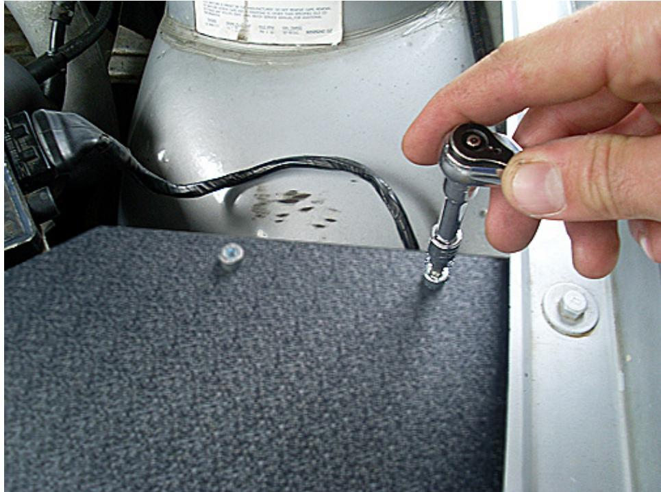
Airbox assembly is now complete. Check the edges around the lid fit nicely with the contours of the car panels. Note that the mounting positions in step 4 of part 3 and the bracket bolts in step 1 of part 3 allow for considerable adjustment. If the airbox does not fit well relative to the car panels, loosen the mounts and the bracket & adjust the box until fit is precise.
