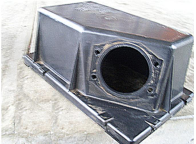
**Step 7** - There are 3 fasteners that fix the base of the airbox to the body. Loosen and remove them
