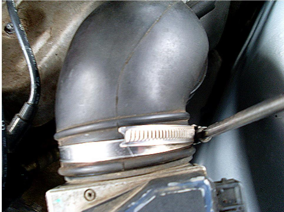
**Step 7** – From inside the enclosure, slide the pod filter onto the adapter & tighten the hose clamp.
