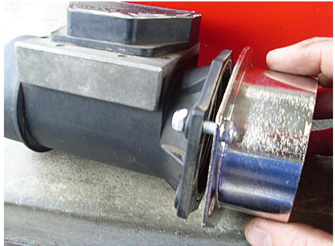
**Step 2** - Tighten the bolts in position.
