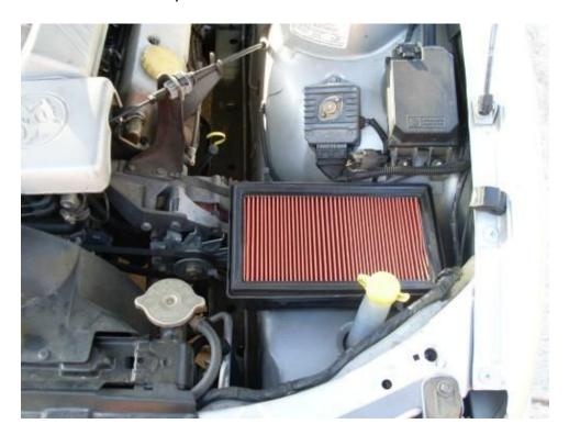
**Step 5** –There are 3 nuts holding the base of the airbox to the car body. Loosen & remove them. The airbox can then be lifted out by hand.
