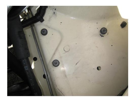
Firstly locate the studs beneath the guard as shown in the image below.
