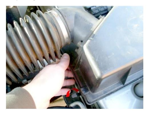
**Step 3**– When all the clips have been released, remove the lid of the air box.
