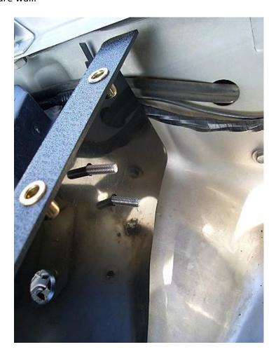
Feed the bracket through the screws, and tighten using flat washer, spring washer & nut.
