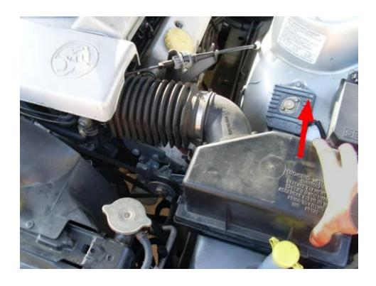
**Step 4** –Lift out the air filter element by hand.
