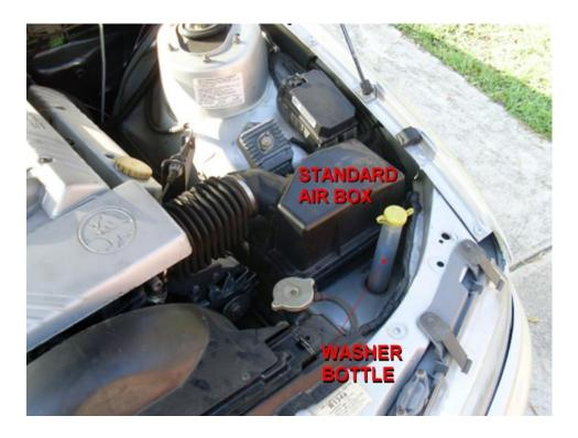
**Step 1** – Loosen the hose clamp of the inlet duct near the throttle body.
