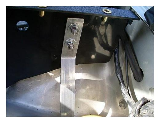
Fasten into the base using an allen key. Make sure to include flat washer & spring washer.
