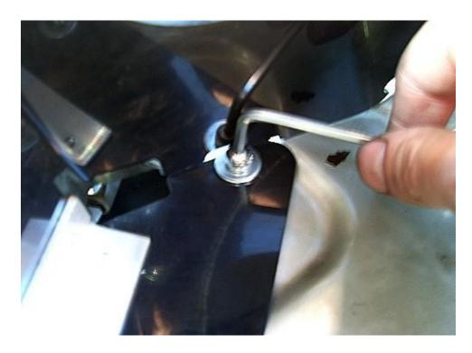
**Step 4** – The support bracket is to be inserted in the following manner. Place the 2 screws through the holes in the enclosure wall.
