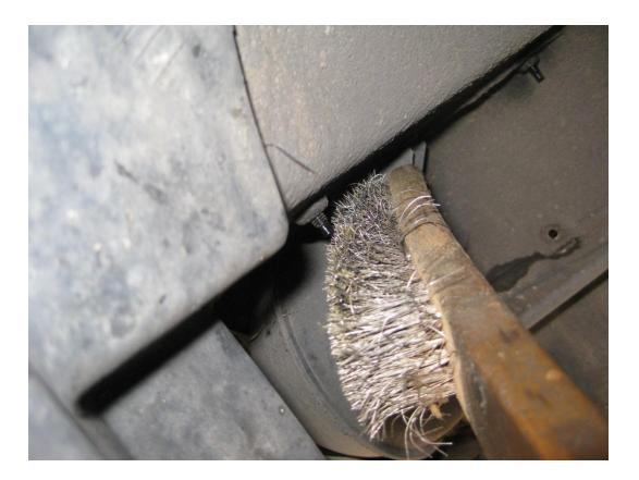
Also spray the top of the studs with the chain lube to dislodge the mating surfaces which may have bonded together due to corrosion.
