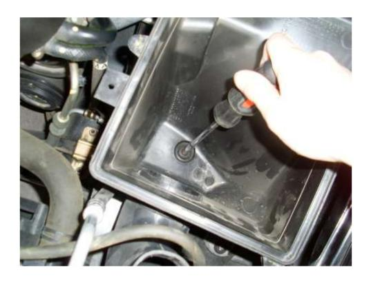
Remove the coolant line from the coolant reservoir by pulling out the rubber grommet as shown below.
