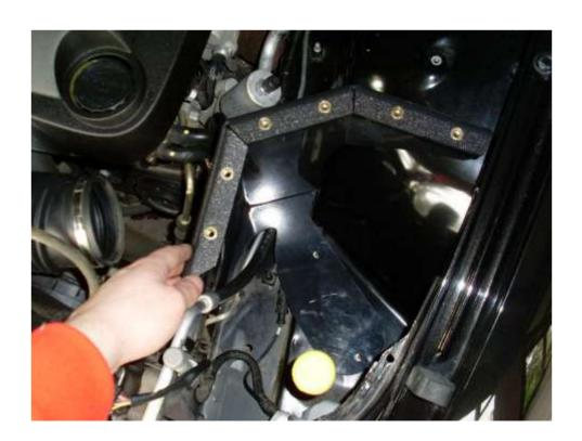
Step 2 – Remove the MAF housing from the old air box lid by undoing the 2 nuts (shown below).
