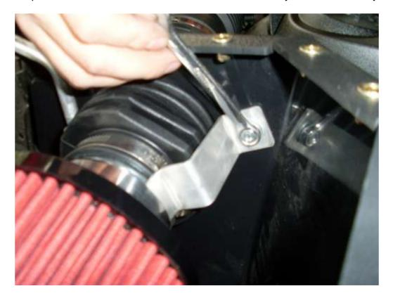
You may need to hold the screw in place while tightening the nut as shown below.
