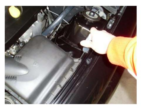
Remove the screws using a Phillips screw driver
