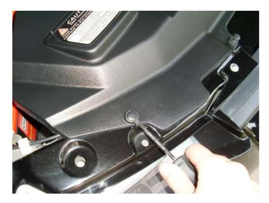
**Step 1** – Carefully wedge a flat headed screwdriver underneath the head of the plastic screw and twist the screwdriver until the clip/screw and be lifted out. There are 5 clips as such. Proceed by removing the radiator shroud which can then be lifted out.
