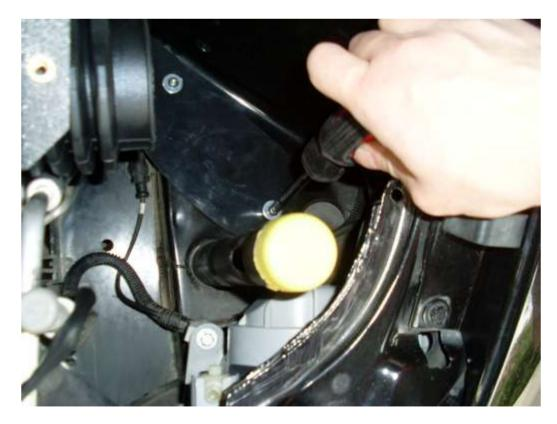
Step 8- Insert the pod adapter pipe into convoluted hose and tighten hose clamp.
