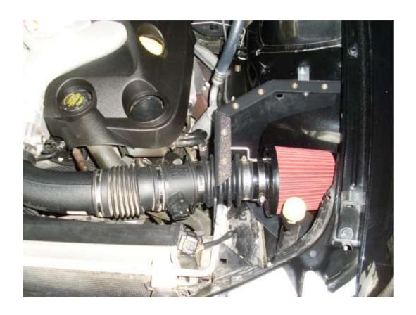
**Step 12** – Refit the MAF plug into the MAF housing.
