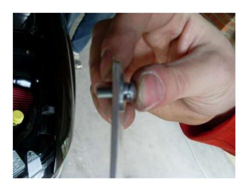
This bracket is used in conjunction with the 3<sup>rd</sup> and remaining original mounting point.
