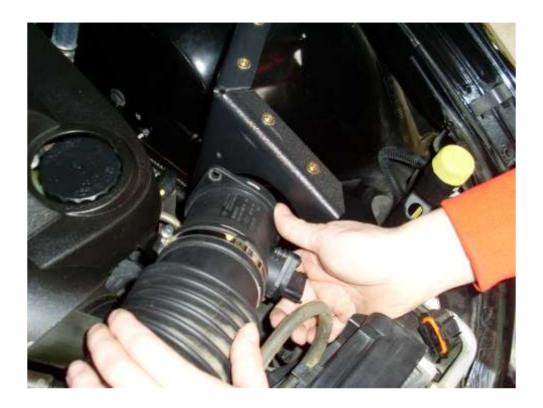
**Step 5** – Place convolute section of intake hose into the hole of the enclosure. The enclosure can be lifted back out of the vehicle if it makes it easier for the installer.
