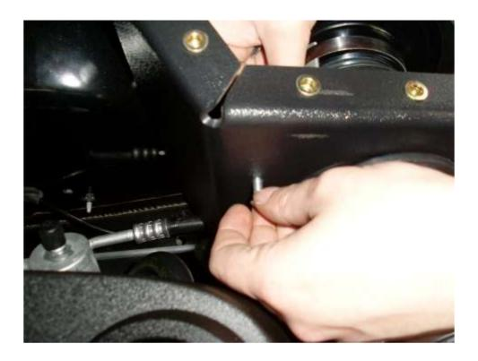
Secure the bracket using a supplied flat washer and nut as shown
