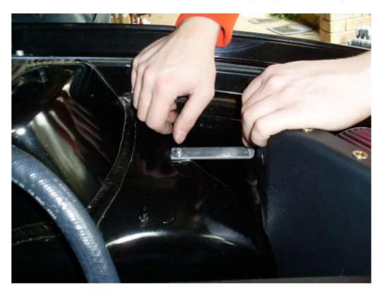
The bracket is secured to the CAI enclosure via a screw, nut and flat washer as shown below.
