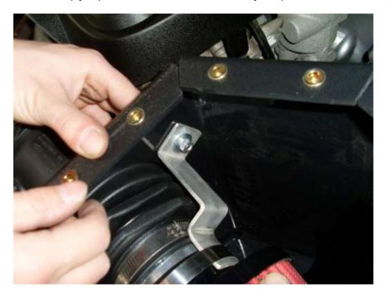
Adjust the position of the POD filter such that it clears the bodywork to avoid any rattles.
