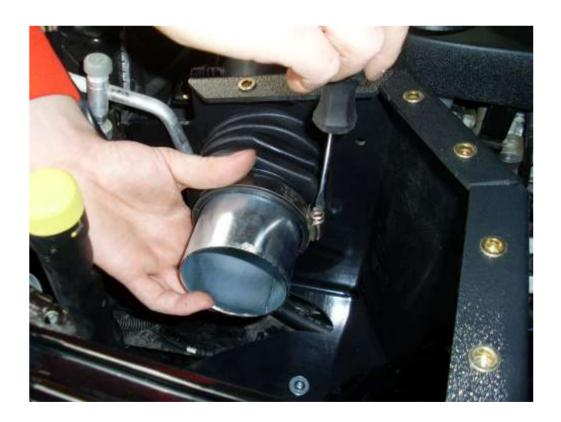
**Step 9** - Slide pod filter over the adapter pipe however do not tighten the hose clamp yet. Please note later on you need to carefully tighten over the adaptor tube such that it doesn't leak between the tube and the hose.
