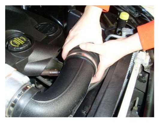
**Step 4 -** Reattach the MAF housing and secure it with the original hose clamp.
