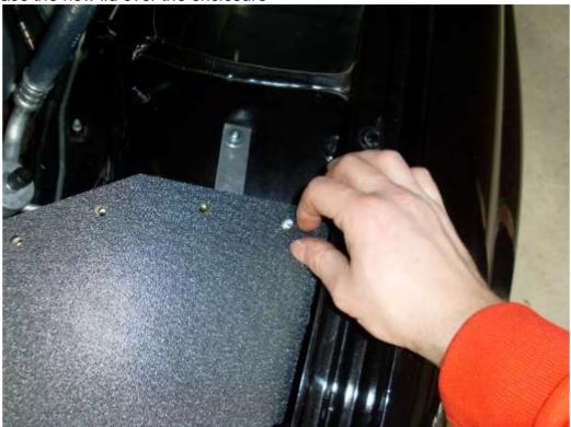
Secure the lid using the 6 screws provided and tighten them using an Allen key.
