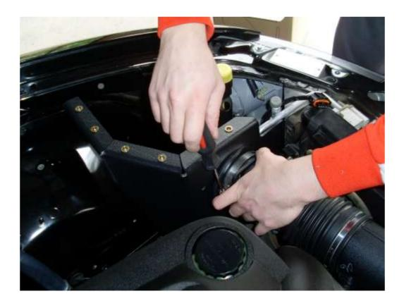
**Step 7** – Secure the CAI enclosure using the bottom 2 of the vehicles original mounting points.
