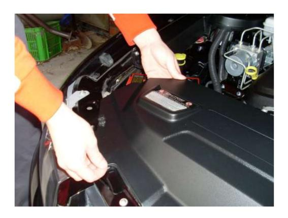
**Step 2** – There are 3 screws which hold the lid onto the air box enclosure.
