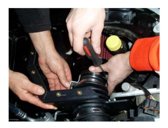
**Step 10** – Place a screw through the hole shown in order to secure the bracket.
