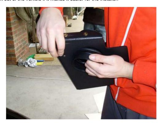
It may be necessary to loosen the hose clamp on the intake elbow such that it can be rotated for proper alignment.
