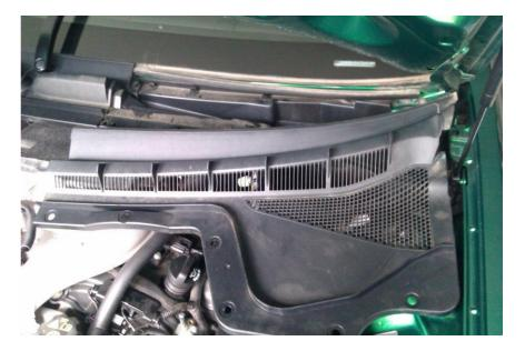
5. Remove the plastic clips on the plastic windscreen trim underneath the rubber trim that was just removed again using a flat-head screwdriver to assist.
