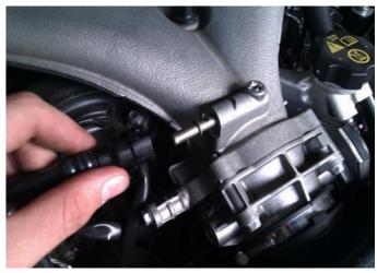
3. Unclip the MAP sensor from the rear left-hand side of the engine.
