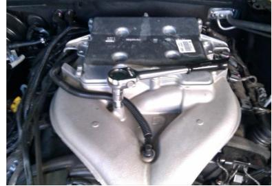
10. Pull intake manifold off by lifting upward and toward yourself (standing at front of the car).
