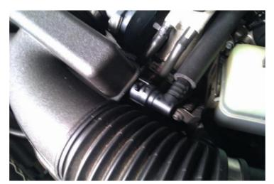
It is removed from the rear of the engine by simply pulling it straight out in and upward direction.
