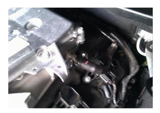
5. Remove the 10mm bolt which attaches a bracket to the left side of the intake manifold.
