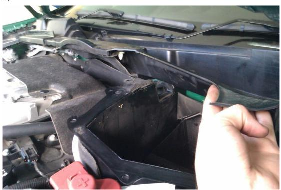
7. Remove the intake manifold cover by removing the two plastic clips on either side with a flat-head screw driver.
