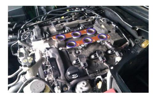
3. Reassemble the manifold in the reverse order
