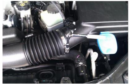
3. Loosen the hose clamp at the front of the MAF sensor. (Again, not all the way off, just enough to remove the intake pipe). Now pull of the intake pipe.
