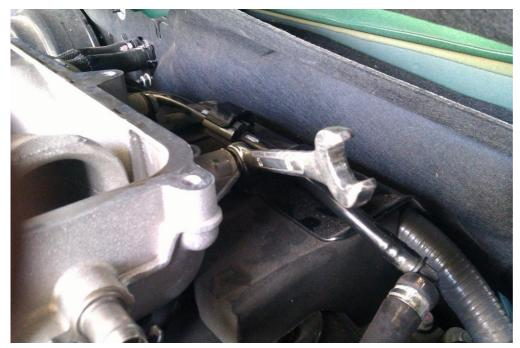
6. Remove the bolts at the rear of the intake manifold using a 13mm spanner.
