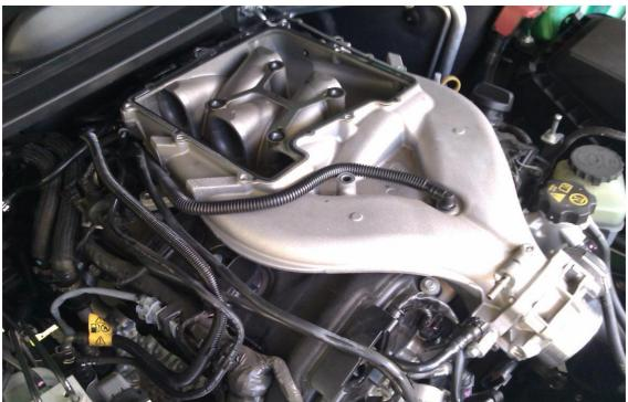
Remove all six (or two, if optional step was completed) 10mm bolts holding the intake manifold in place.
