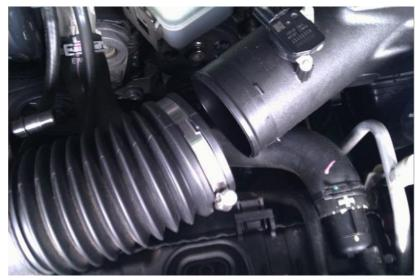
4. The complete intake piping should now be removed leaving the airbox in its position.
