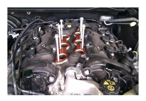
2. Also apply sealant on the **upper side** of the insulators as shown below.
