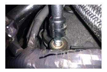
\*To assist in the rest of the installation ask a friend to hold up the windscreen trim or retain the windscreen trim yourself with something (eg. Screwdriver) to hold it up. This gives more room behind the intake manifold to work.
