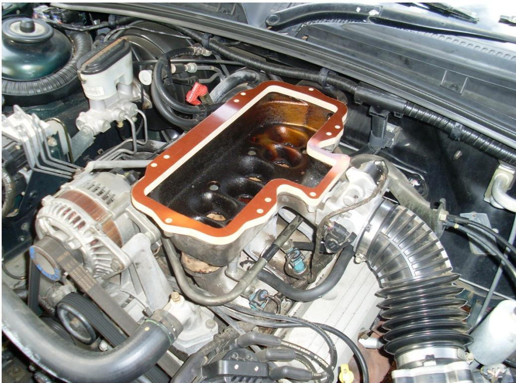
**Step 5** – Place a secondary layer of gasket maker onto the surface of the plenum spacer.
