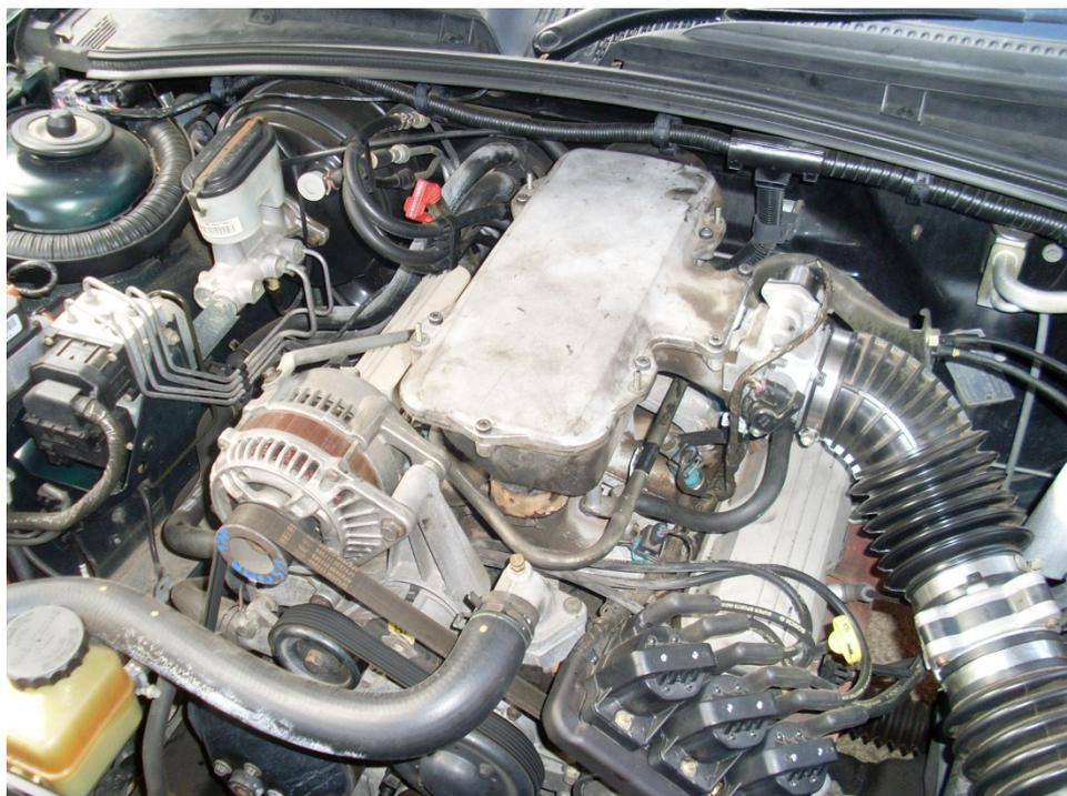
**Step 2** – Locate the 7 socket headed bolts which retain the plenum cover. The location of the bolts is shown below.
