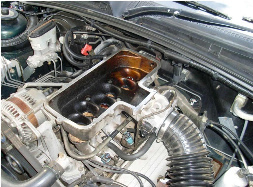
**Step 3** – Place an even amount of about 3-4mm of gasket maker onto the plenum face as shown.
