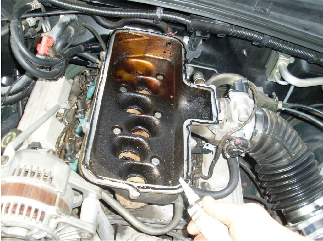
Place the plenum spacer onto the plenum as shown. The plenum spacer is symmetrical across the horizontal axis and will fit the plenum either way.
