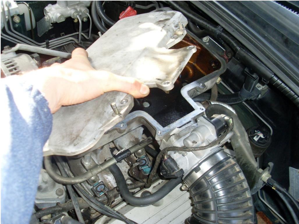
Remove old gasket and any debris using a scraper and/or wax remover if necessary.
