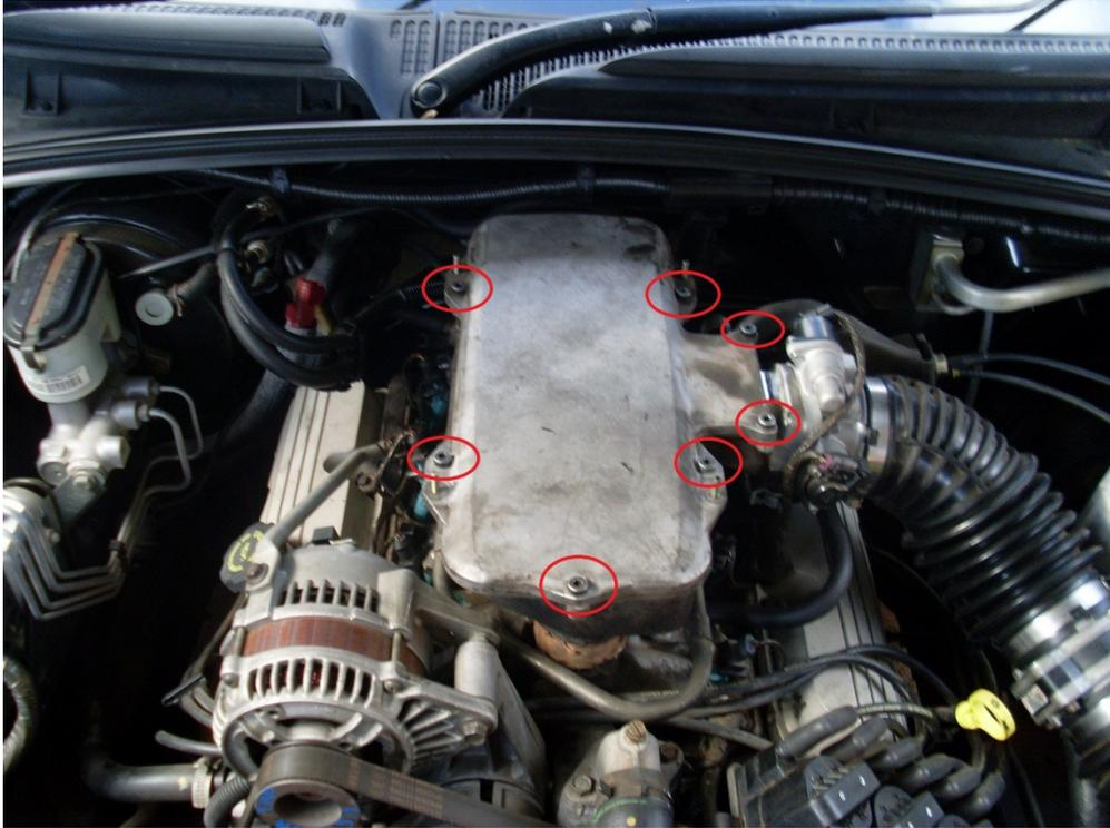
Unfasten the bolts using an Allen key
