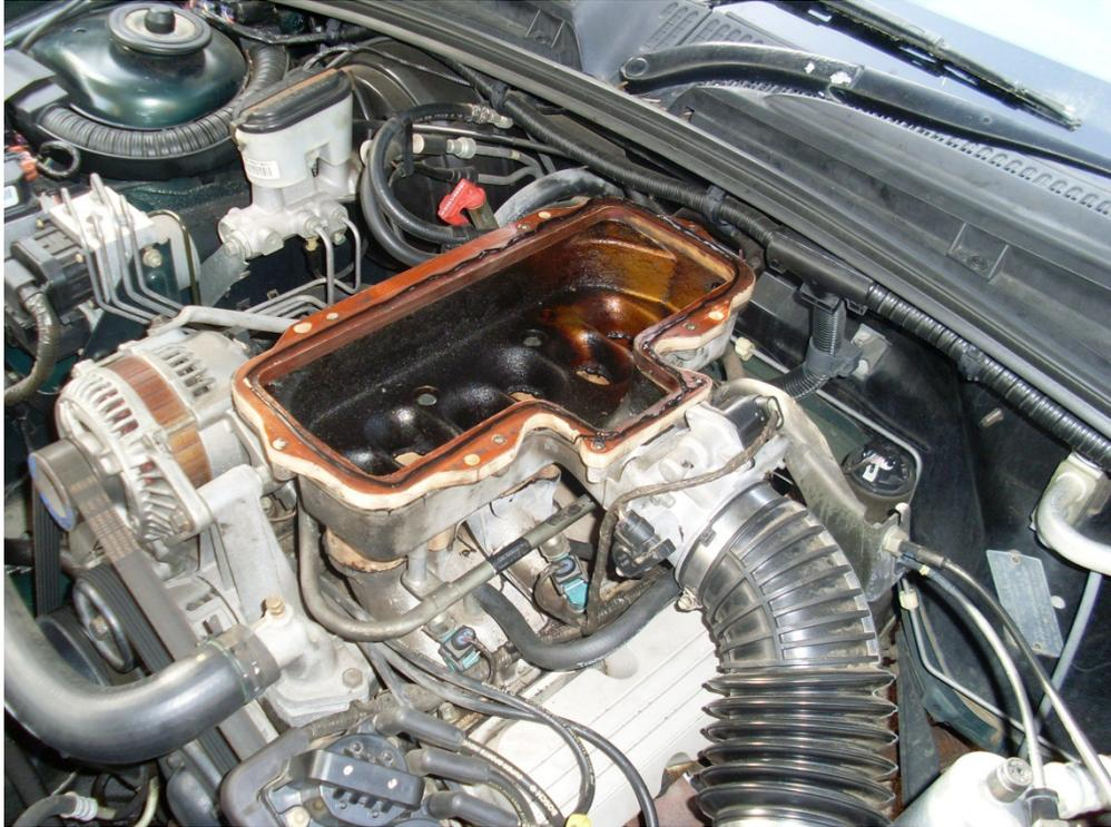
Fit the plenum cover onto the plenum spacer and tighten all bolts as shown. It is recommended to torque the bolts to 13-16 Nm using a torque wrench.
