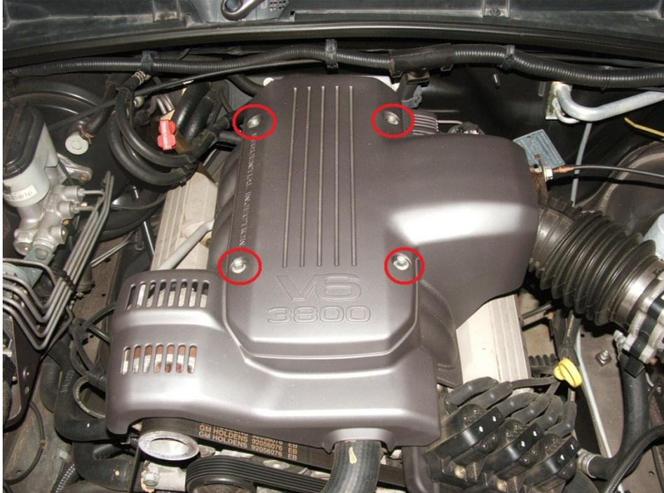
The engine cover can then simply be lifted off the engine
