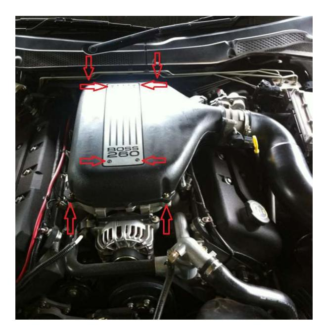
Once the four inner bolts are exposed they can be easily removed.
