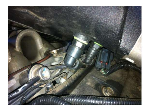
Complete the plenum removal by disconnecting the three electrical connections (TPS, MAP and throttle) and taking the main brake line off the back of the plenum.
