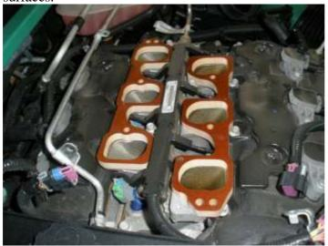
**Step 3:** Spread the gasket sealant provided with the kit around the surface of each runner. Do not spread gasket sealant around the bolt holes.
