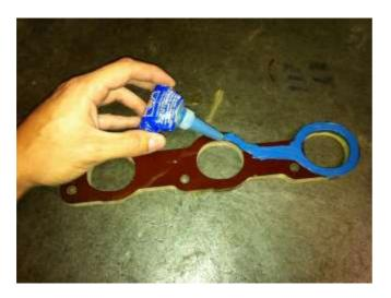
(Picture is to be used as a guide to illustrate how to spread the Silicone over the Manifold Insulator)
