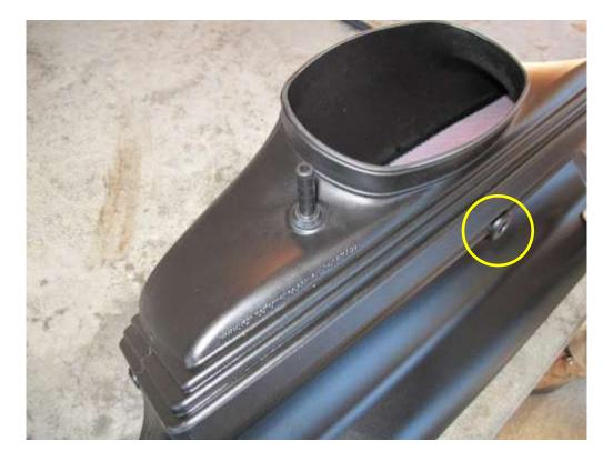
Insert the drain valve into the bottom central hole of the OTR.
