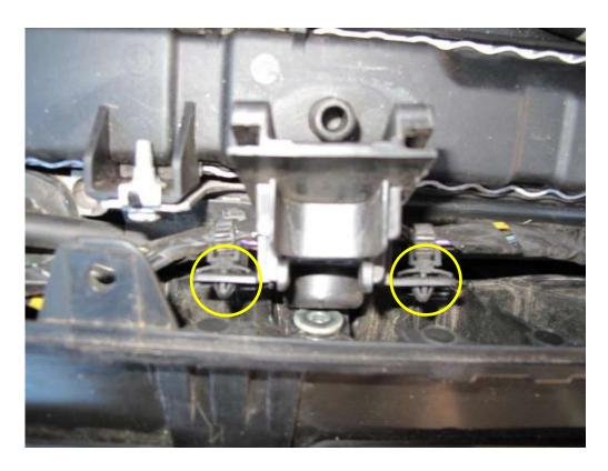
• Using a pair of pliers, release the lower support from the wiring loom from both the lower radiator support bracket.
