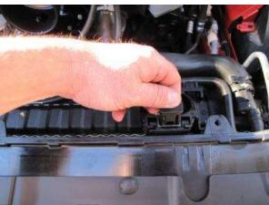
• Remove the radiator support locking wedge from both sides.
