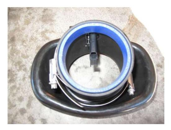
• Fit the coupling to the MAF housing as show and tighten only the coupling worm drive hose clamp, leaving the other end loose to fit on to the throttle body.
