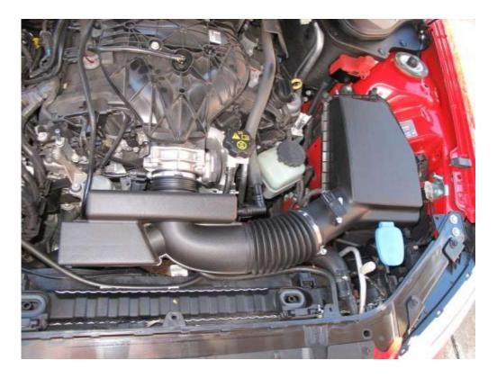
To remove the factory air intake, begin by disconnecting the MAF and vacuum sensors (Circled below) by pushing down on the locking tab before gently pulling the loom away from the sensor.
