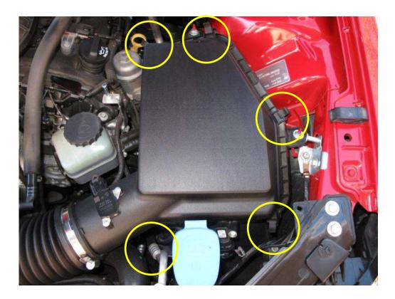
• Unclip the top of the factory air box top cover, circled above and below. This can be achieved by hand and requires no tools.
