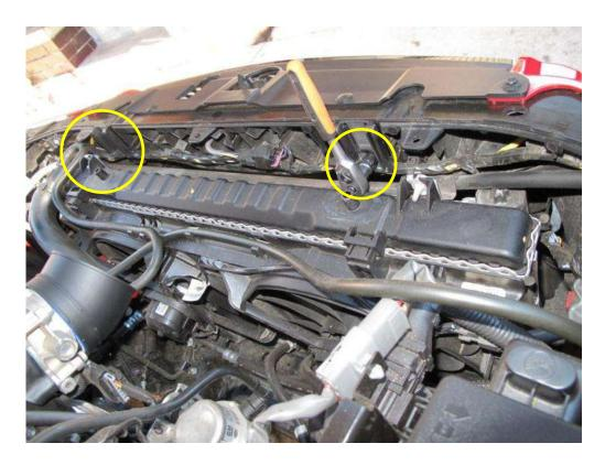
• Remove the 10mm screws holding the lower part of the radiator support bracket from both left and right side and reserve for mounting the leaning bracket supplied in the VCM kit.
