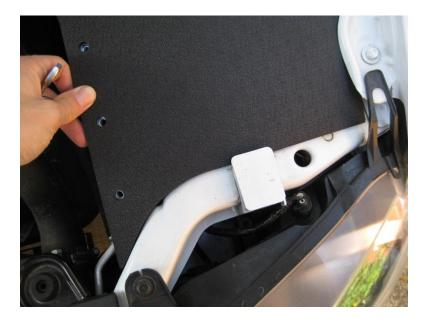
Secure the lid buy screwing in the 6 remaining cap screws with an Allen key.
