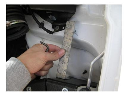
Install a 6mm socket-headed cap screw (longer side of bracket) with an Allen key placing both a spring and flat washer beneath it. The spring washer is installed closest to the screw head.
