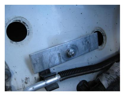
Slide in the enclosure with correct orientation and tighten the nut such that the bracket is secure.
