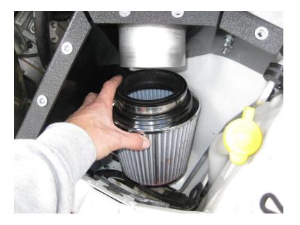
Tighten the hose clamp to ensure the pod filter is secure.
