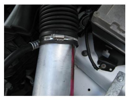
Once inserted approx. 15-20 mm, tighten the hose clamp to ensure the pipe is secured.
