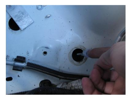
Insert the end of the screw through the hole.
