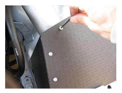
In order to achieve perfect alignment some adjustment may be required. This can be achieved by loosening all brackets and screws and holding the enclosure in place and retightening the screws.
