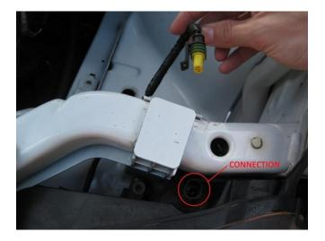
Remove the plastic screw holding the loom's cabling in place on the inside of the radiator support.
