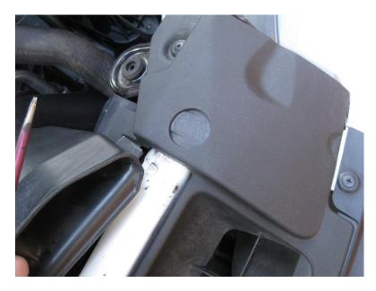
The snorkel also connects to the factory air-box and can be simply removed by rotating away from the engine and sliding it off the air-box pipe.
