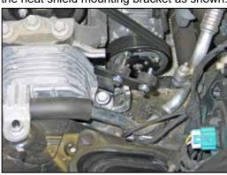
9. Install the heat shield mounting bracket onto the motor mount and secure with the factory bolt removed in step #7.
