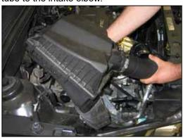
5. Lift the airbox assembly to dislodge it from the mounting grommets and then remove the airbox from the vehicle.
