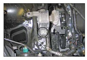
7. Remove the front motor mount bolt shown. **NOTE: This bolt will be reused in a later step.**
