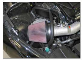
17. Install the K&N<sup>®</sup> air filter onto the filter adapter and secure with the provided hose clamp.
