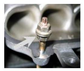
You are now ready to remove the guide pin. Use the 10mm open ended wrench on the bottom nut to unscrew it. For easy alignment, leave the two 4mm guide pins in but loose so that they can be removed after the plenum top is lowered.
