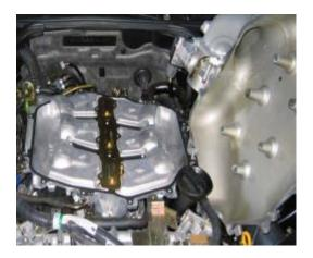
Use a paper towel and degreaser to wipe up any dirt and oil. Clean the top, bottom and around the edges to remove any debris and residue. The interior of the plenum may be very oily but this is normal and OK. You can leave the stock gasket in place but you can take it out too. Either way, the plenum will still seal. It would be good practice to leave the stock gasket in place in the event you decide to sell the car and keep the spacer.
